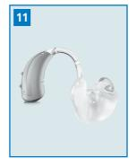
Curve of the ear mould should line up with curve of the hearing aid.
