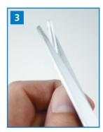
Cut end off new tubing into a taper.
