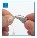
Secure the LifeTip to the ThinTube. Carefully screw the ThinTube to the hearing aid to reconnect.
